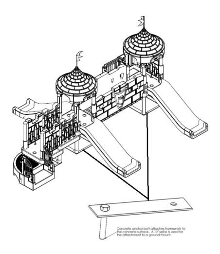
Secure structure to solid surface using anchor bolts, or secure structure to ground using  $0.47 \times 0.98$  in spikes. (Not provided)
