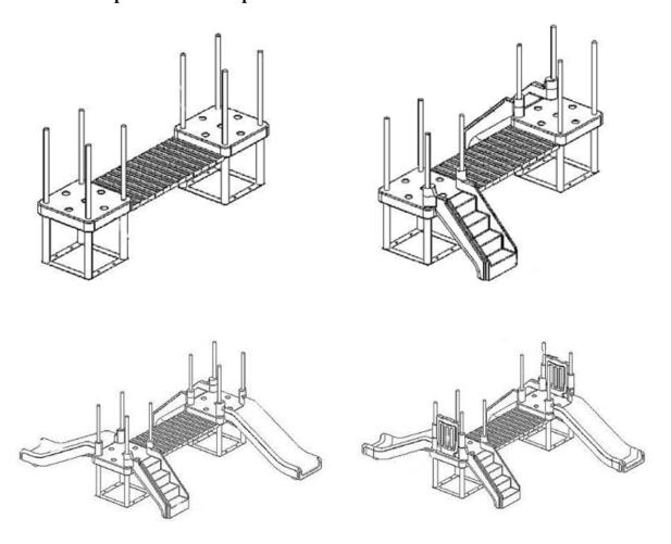
Place all the panels over the posts including the castle bridge walls and handrail of stairs and drill a  $\emptyset$ 0,46in hole through post where stair handrail will attach. Attach stair handrails with hardware provided.
