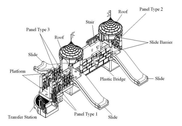
Set up main frames so that the longer posts face inwards. Slide the bridge support pipes through the twelve plastic bridge segments and insert bridge supports into pre-drilled holes in the main frames.
